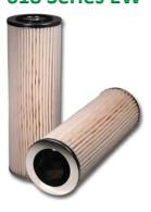
PetroClear models PCP-E10 and PCP-E30 are particulate removing replacement element type filters designed to remove particulate (dirt) from Neat Gasoline, Ethanol Blended Gasoline, Diesel, Biodiesel, ULSD (Ultra Low Sulfur Diesel), Kerosene, Fuel Oils, Lube Oils and Synthetic Fluids. These filters are designed for particulate removal only and will NOT react to water in Neat Gasoline or detect Phase Separation in Ethanol Blended Gasoline.
