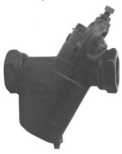
Y-type strainer used in pipelines to filter debris from flowing into and damaging equipment such as a pump or a meter. Strainer basket is removable for cleaning and/or replacement.
